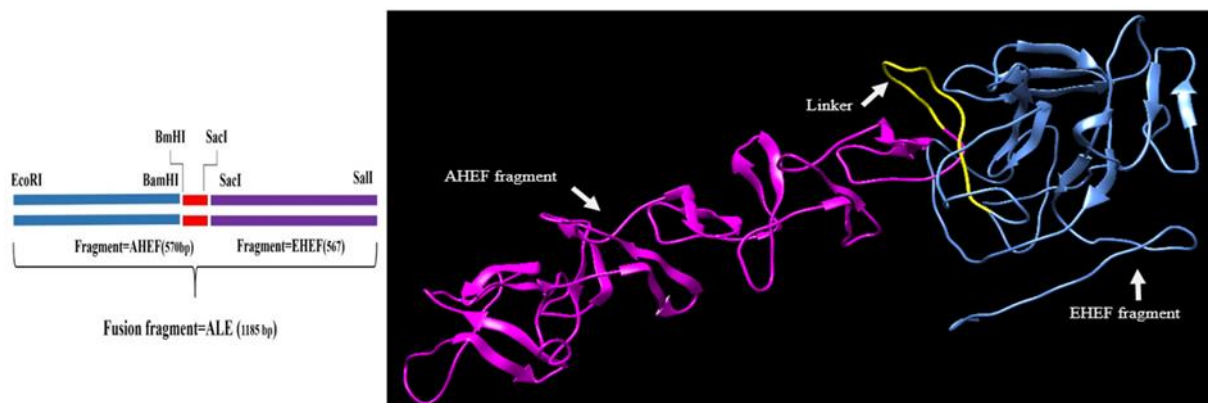
Figure 2. Schematic 3D representation of the designed fusion protein as it was drafted by the I-Tasser .... (A). Restriction map of the recombinant protein ALE (B). Different enzymes including EcoRI, BamHI, SacI, and Sall were applied to connect desirable fragments. The Linker was restricted by BamHI and Sall. In the final structure, AHEF (alpha toxin related fragment: pink-colored structure) is bounded to the EHEF (epsilon toxin related fragment: blue-colored structure) via the yellow-colored linker.
